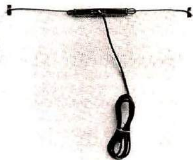
A paste-on DF antenna that can be fastened to an airplane windshield makes an easy and effective temporary installation. Note phasing line in the center.
