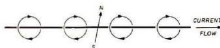
Fig. 3. A current (electron) flow through a wire sets up a magnetic field around the wire. If you grip the wire in your left hand, with your thumb pointing in the direction of current flow, your fingers curl around the wire in the direction of the north pole of the magnetic lines of force. A compass placed on the wire will indicate the lines of force by aligning its pointer with the field, at right angles to the wire.
