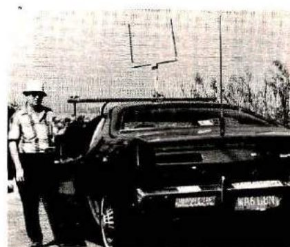
Andy Memmel, WA6CBN, stands beside his car, which has been fitted with a demountable roof rack containing a pulley system that allows him to change antenna direction and read azimuth bearings from the driver's seat.
