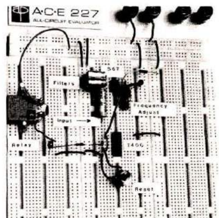
Breadboard layout of the latching flip-flop circuit shown in Fig. 4.
