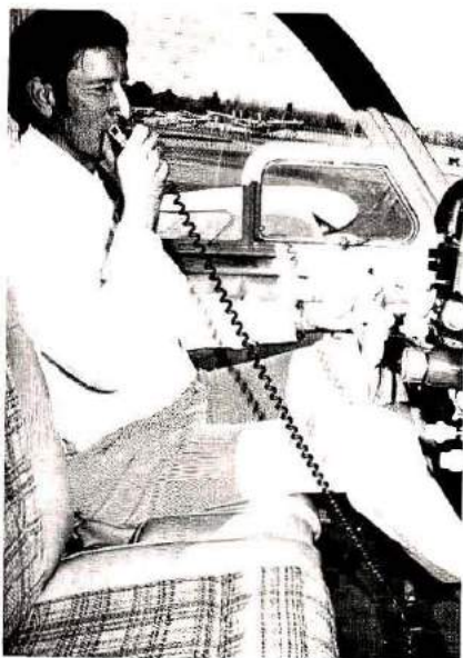
Bill Cryer, W6RCC, at the controls in his Bonanza airplane. Equipment includes low-band and vhf radios. A longwire antenna can be extended from the back of the airplane in flight. An ICOM 230 radio is used for vhf.
